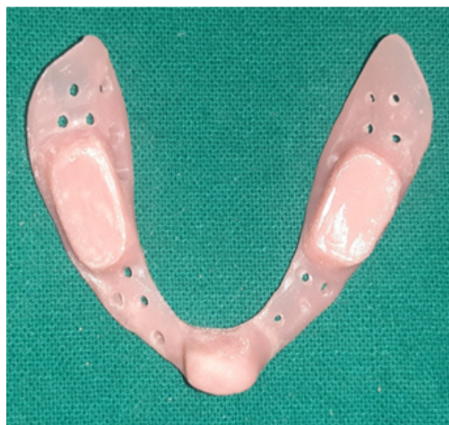
Fig. 3: Perforated acrylic custom tray with two stub handles
